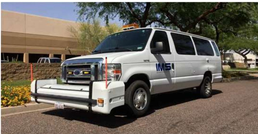
**Figure 4 – Laser Road Surface Tester (RST)**
