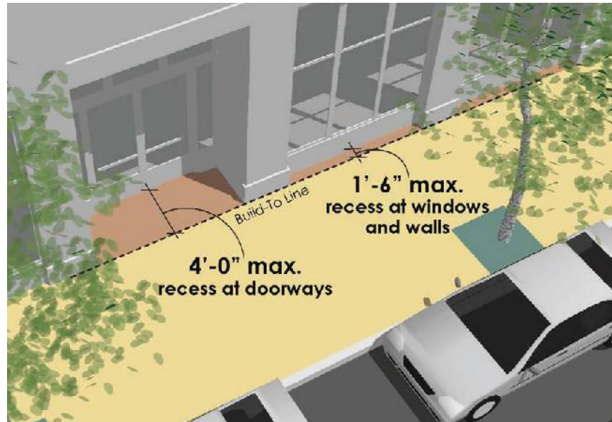
Figure 18.606.110.A.3 Recessed Entries and Windows for Zero Setbacks [Image: Crandall Arambula]
